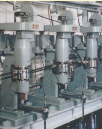
Fig. 1-3 Rolling fatigue life test conditions and test equipment
